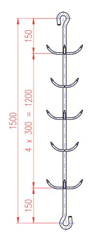
The fresh meat tree is used for meat hanging and transport on the flat-bar or roundbar railways. Carrier bar is finished with loop on both sides on which is the hook hanged on hook for flat-bar railway or sliding hook. The meat is hanged on little hooks which are welded to the carrier bar. The whole product is made of stainless steel.
